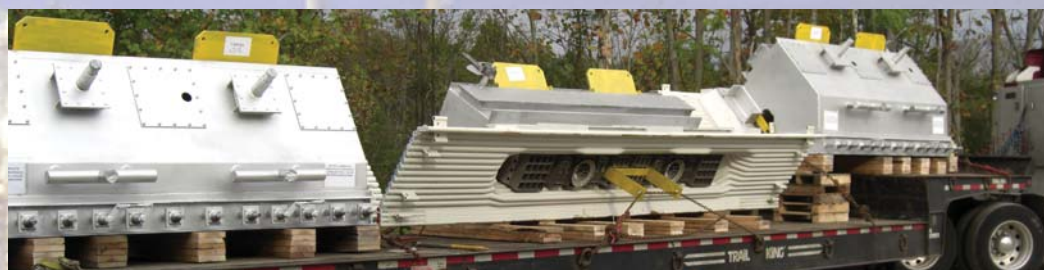
Complete Windbox Assembly w/Shop Mounted Tube Panel
