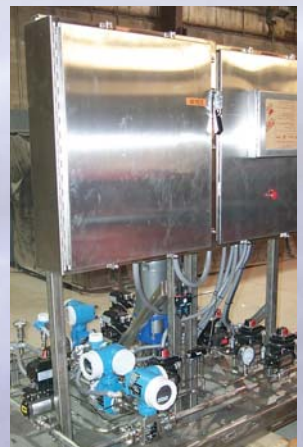
Urea Skid w/Shop Wired Controls
