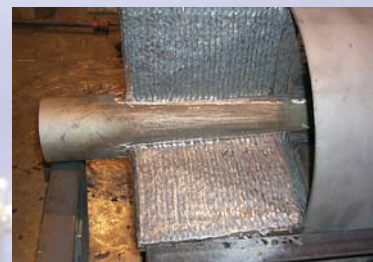
Round Burner Coal Spreader w/Overlay
