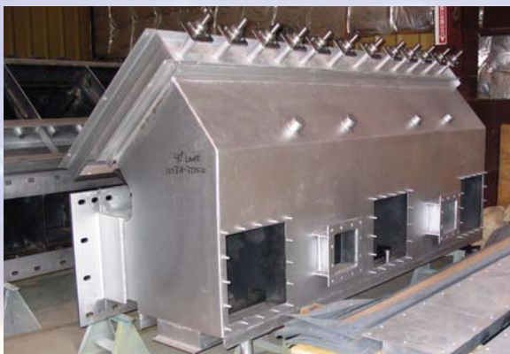
Wind Box Assembly During Fabrication
