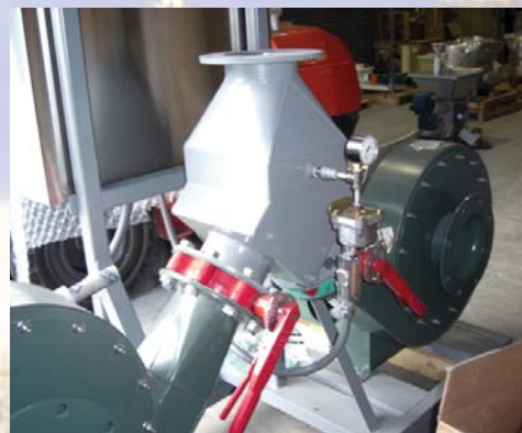
Fan Skid with Diverter Damper and Operator
