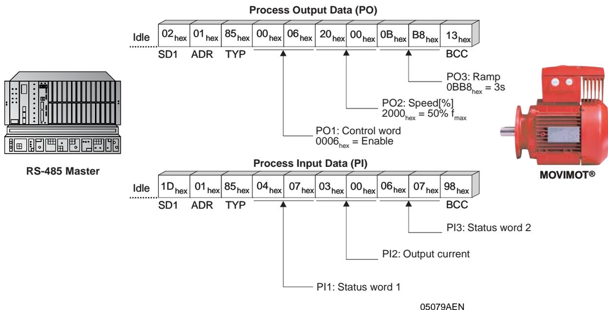
This example shows acyclical transmission, i.e. no timeout monitoring is active in MOVIMOT<sup>®</sup>. Cyclical transmission can be implemented with the entry TYPE = 05<sub>hex</sub>. In this case, MOVIMOT<sup>®</sup> expects the next bus activity (request message of the aforementioned types) within one second at most, otherwise MOVIMOT<sup>®</sup> automatically brings itself to a stop (timeout monitoring).
