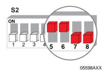
The current limitation can be set via switch f2. The binary input terminal f1/f2 can be Function descripused to toggle between maximum current limit and the current limitation set via switch f2. tion
