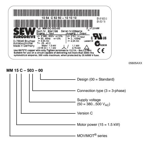
The device identification [1] at the top of the MOVIMOT<sup>®</sup> inverter contains information Device identification about inverter type [2], inverter part number [3], equipment power [4] and adapted (associated) motors [5].
