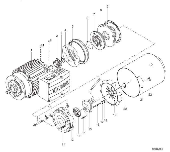
Motor with brake end shield 1
