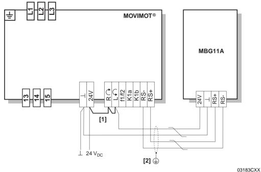
Observe the enabled direction of rotation (see the section "Connection of MOVIMOT<sup>®</sup> basic unit, Functions of CW/Stop, CCW/Stop terminals with control via RS-485 interface.")
