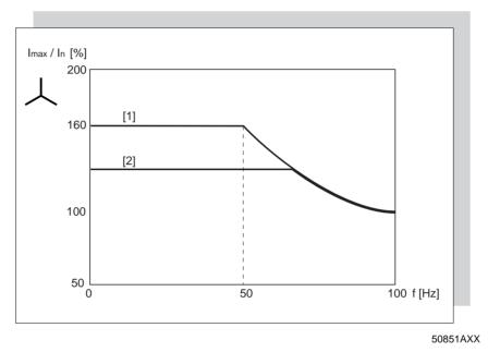
[1] Current limit characteristic curve of standard function
