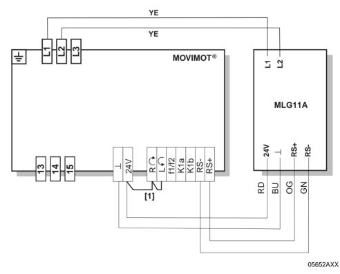
Observe the enabled direction of rotation (see the section "Connection of MOVIMOT<sup>®</sup> basic unit, Functions of CW/Stop, CCW/Stop terminals with control via RS-485 interface.")
