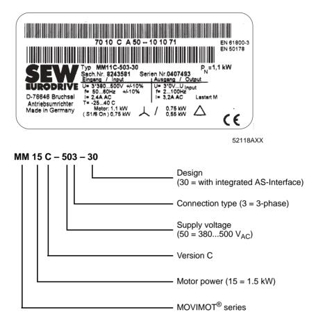
*Device identification* The device identification [1] at the top of the MOVIMOT<sup>®</sup> inverter contains information about inverter type [2], inverter part number [3], equipment power [4] and adapted (associated) motors [5].
