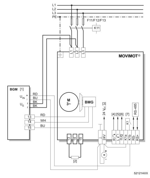
[1] Brake control BGM installed in the terminal box
