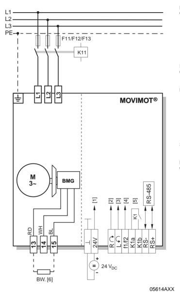
Function of terminals CW/Stop and CCW/Stop with binary control:
