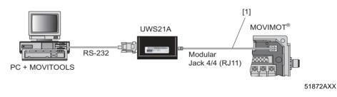
[1] Feed the cable through the cable entry into the MOVIMOT<sup>®</sup> wiring space!
