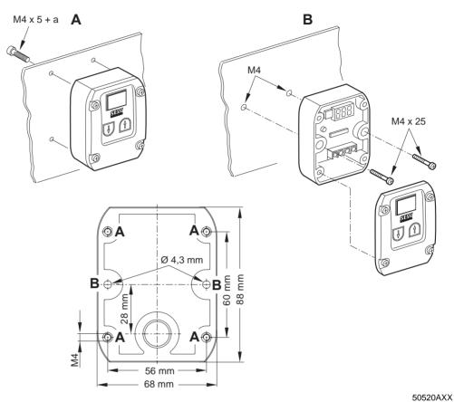
a = wall thickness Screws are not included in the delivery!
