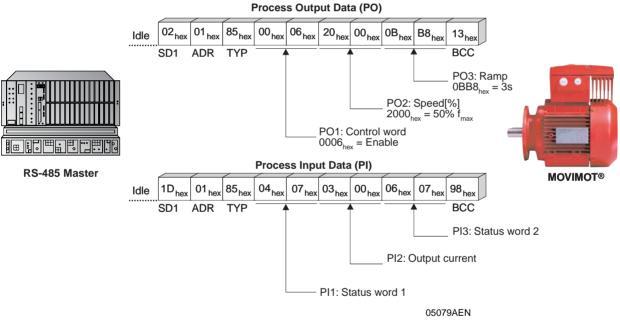
This example shows acyclical transmission, i.e. no timeout monitoring is active in  $MOVIMOT^{\$}$ . Cyclical transmission can be implemented with the entry TYPE =  $05_{hex}$ . In this case,  $MOVIMOT^{\$}$  expects the next bus activity (request message of the aforementioned types) within one second at most, otherwise  $MOVIMOT^{\$}$  automatically brings itself to a stop (timeout monitoring).
